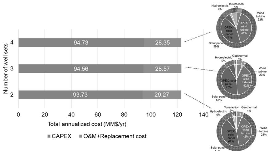
Figure 4: Techno-economic analysis results of the optimal solution for different numbers of ESH well-pairs
