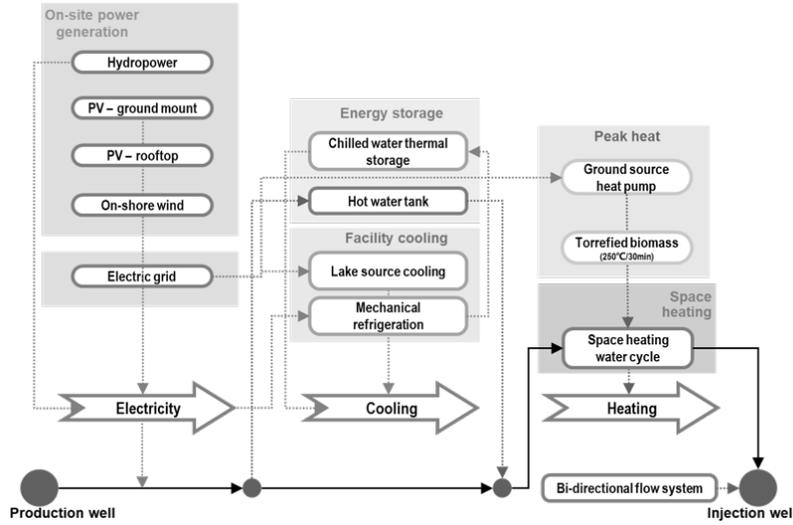
Figure 2: Optimal configuration of campus energy systems
