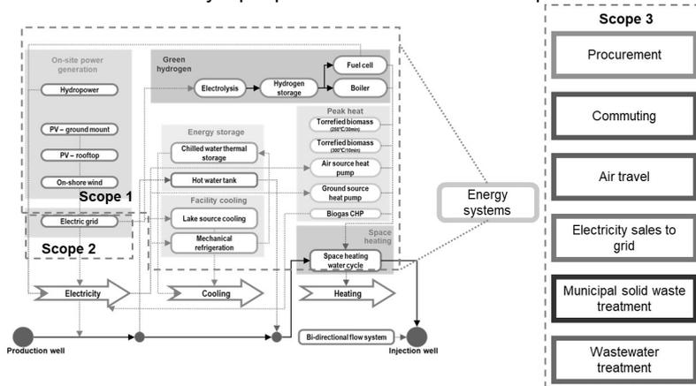
Figure 1: Expanded systems boundary where the scope 1, 2, and 3 are shown in the dotted-line boxes
