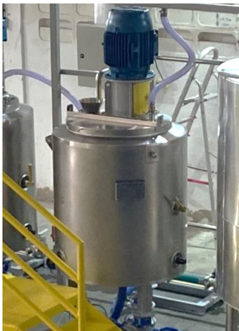
Figure 1: Mixer with a capacity of 250 liters for the biodetergent production process
