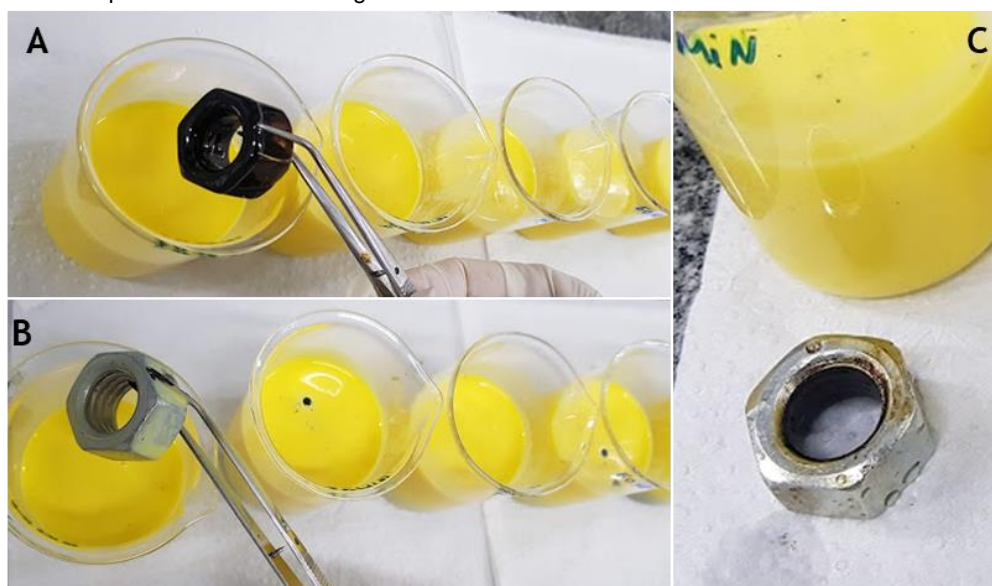
Figure 6: Illustration of the removal of OCB1 oil by the biodetergent on a metallic surface. Metal part impregnated with OCB1 oil (A). Removal of OCB1 after immersion in formulation (B). Oil removal from finished metal surface (C)
