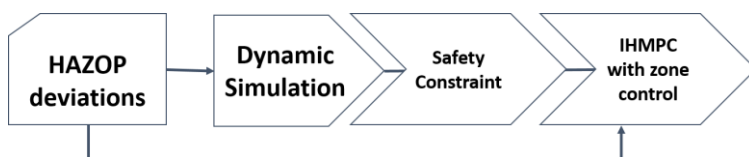
Figure 1: Flowsheet for development of MPC with safety constraint embedded in HAZOP
