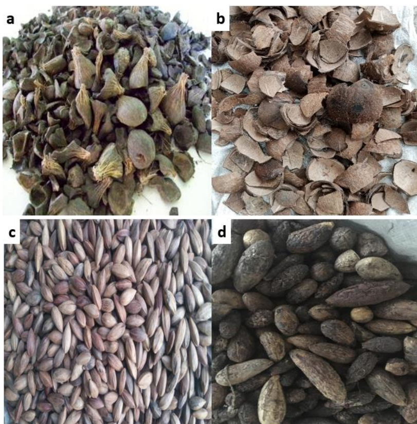
Figure 1: Biosourced materials: a) palm kernels shells, b) coconut nucifera shells, c) canarium schweinfurthii fruit cores and d) fruit cores of raffia vinifera
