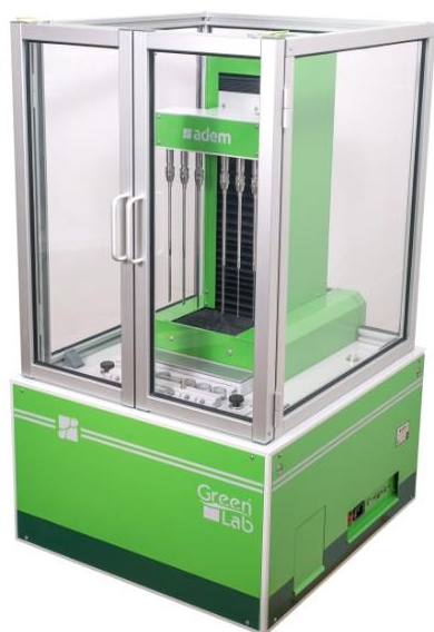
Figure 1: The automated demulsibility tester (ADEM)
