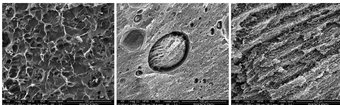
Figure 3. SEM micrographs of PVA2kC4 unirradiated (0 kGy) (A), irradiated at 10 kGy dose (B) and irradiated at 40 kGy dose (C).
