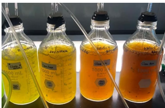
Figure 3. Microalgae using dilution of vinasse as a culturing medium.
