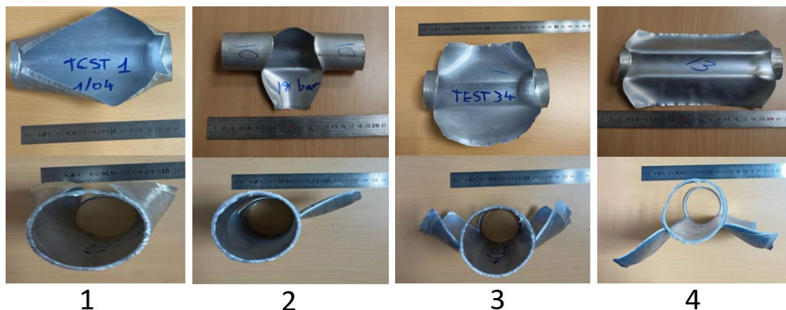
Figure 3: Types of failure front/side view (1). Fish mouth (2). Asymmetrical (3). Incomplete (4). Total opening
