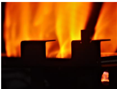
Figure 2: Premixed \text{H}_2 flame with flashback. Figure 3: CBS diffusion \text{H}_2 flame with mesh flame stabiliser.
