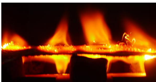
Figure 2: Premixed \text{H}_2 flame with flashback. Figure 3: CBS diffusion \text{H}_2 flame with mesh flame stabiliser.
