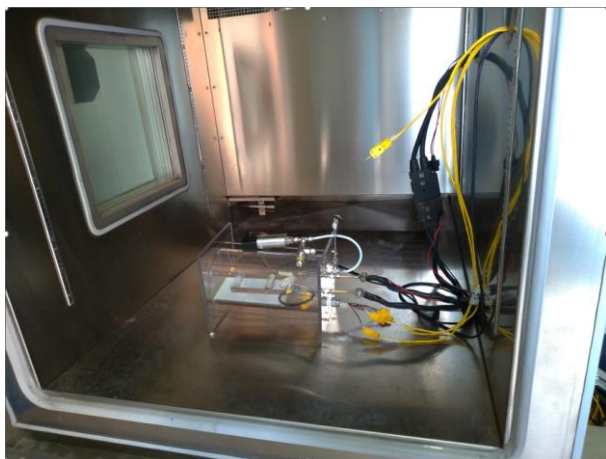
Figure 2: Climatic Chamber with cell container.
