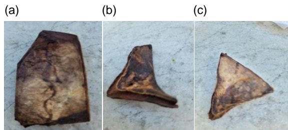
Figure 3: Sample sizes used for determining the initial moisture content of CPH a) large, b) medium, and c) small
