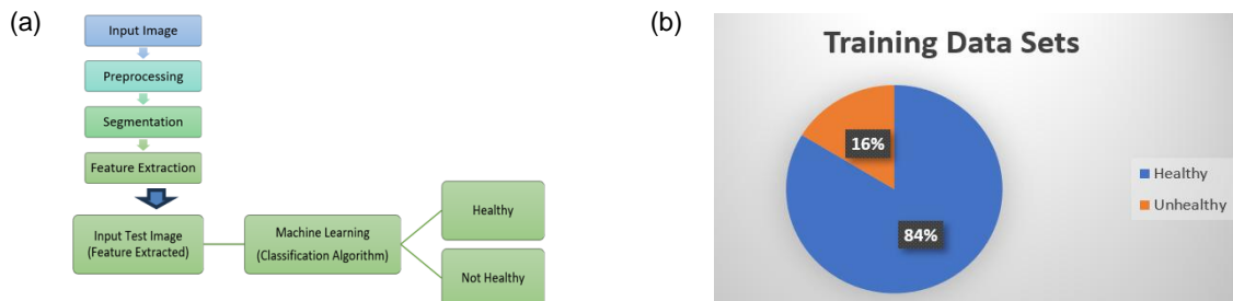
Figure 2: (a) System architecture for the image processing, (b) Training data sets used (3480-healthy, 840-unhealthy)
