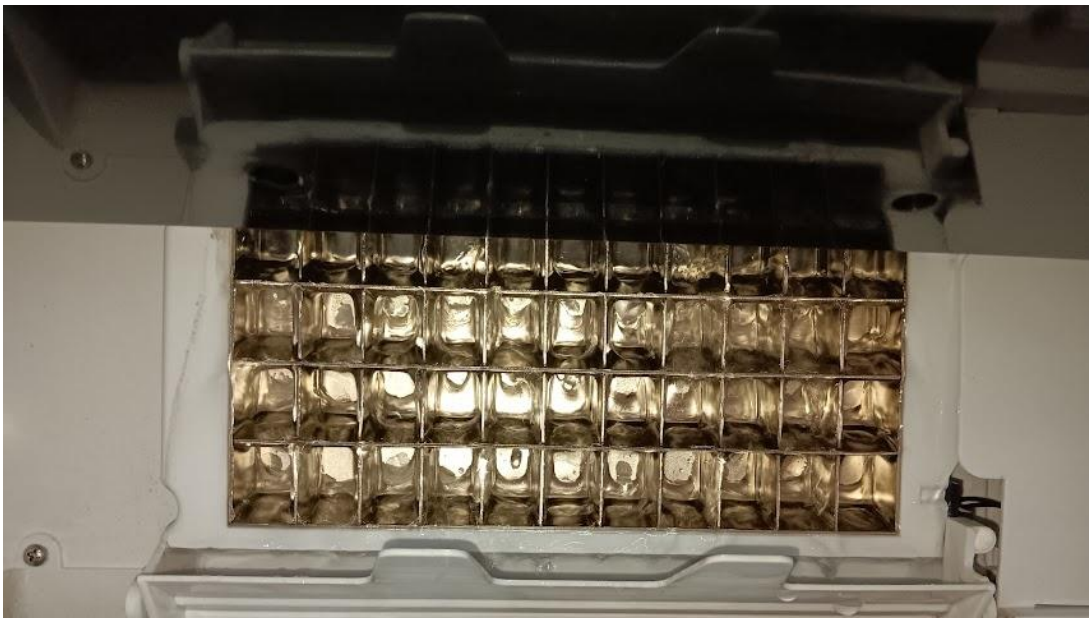
Figure 3: Ice formation in falling-film PFC experimental setup
