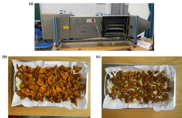
Figure 1: (a) Computer Controlled Tray Drier and turmeric rhizomes; (b) before; (c) after drying process
