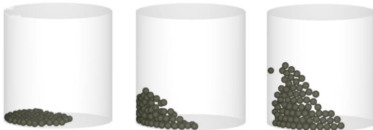
Figure 4: Ball movement inside the mill at different speeds. a) 100 rpm. b) 300 rpm. c) 500rpm
