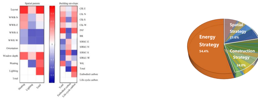
(a) Spatial and construction strategy correlation (b) Distribution of carbon reduction potential of different strategies
