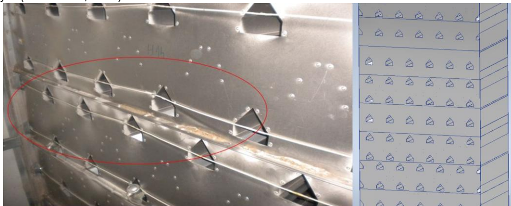
Figure 7: Uneven distribution of air ducts on the surface of the dryer (left) and the 3D model (right)
